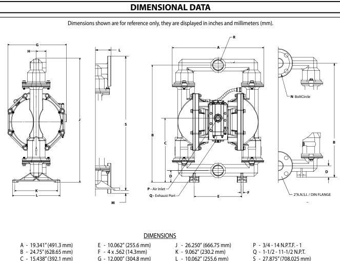
C - 15.438" (392.1 mm) G - 12.000" (304.8 mm) L - 10.062" (255.6 mm) S - 27.875" (708.025 mm) D - 2.500" (63.5 mm) H - 2 x 2.088" (53.03mm) M - 0.600" (15.9 mm)
